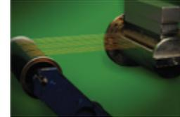
Insulating multiple wire paths with a polymer insulation applicator.
