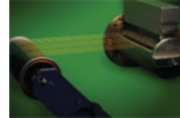
Insulating multiple wire paths with a polymer insulation applicator.
